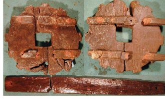
(a) photos of the fractured fountain parts
