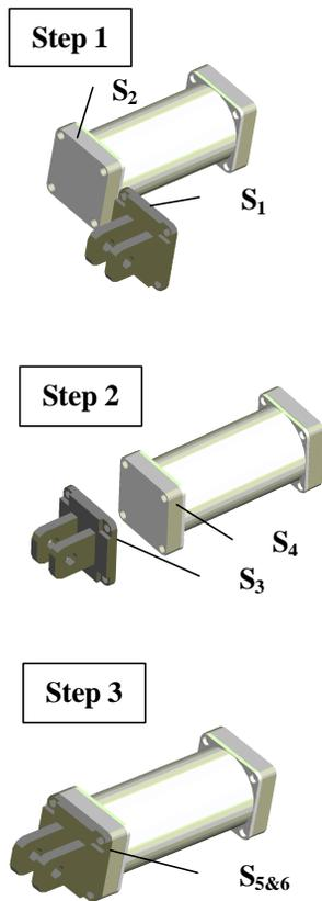
Fig. 9: Assembly operations for CAD parts
