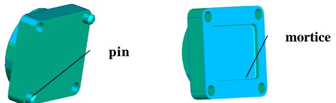
Fig. 10: New design for the clevis mounting part
