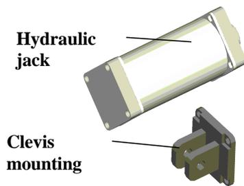
Fig. 8: Hydraulic jack and clevis mounting CAD parts
