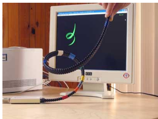
Figure 2. The ShapeTape used as an input device for piloting its 3D virtual copy.
