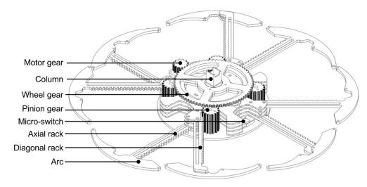
Figure 9: The CAD model of the mechanism of the final expandable ring<sup>6</sup>, designed with OnShape, a Cloud CAD Software.
