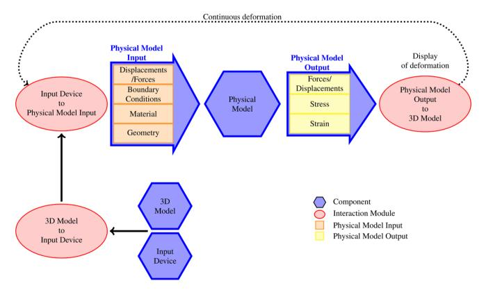
Fig. 1 An illustration of the design principles for a tangible user interface dedicated to physically-realistic deformation
