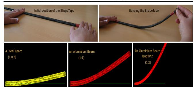
**Fig. 3** A physically-based beam bending, controlled interactively by the ShapeTape. For the same tape displacement, the physical behavior of the beam changes according to the material (steel, aluminum) and
